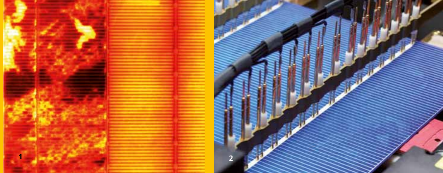
1 Quantitative photoluminescence imaging of solar cells: dark saturation current image (left) and series resistance image (right). 2 Automated IV-curve measurement at PV-TEC.
